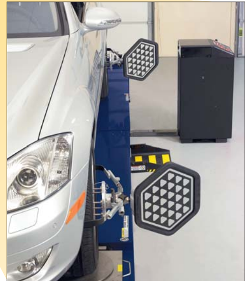
Lightweight durable targets are easy to install.
