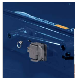
MKS Alignment Sensor Brackets and Harting Rack Wiring Box
