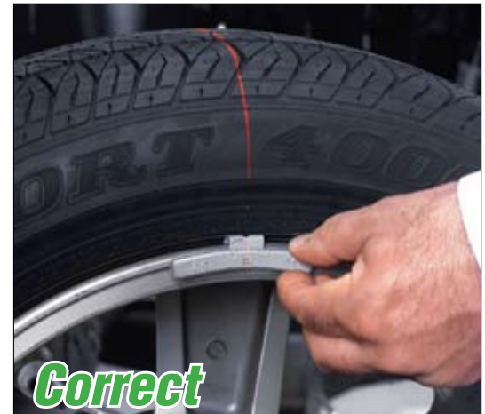
Precision wheel weight placement is fast and easy using the HammerHead TDC laser as a guide.
