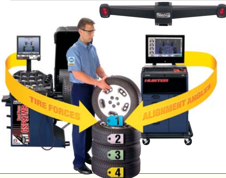
Tires are tagged and positioned on the vehicle to provide the least amount of vehicle pull and obtain the best straight ahead steering stability.
