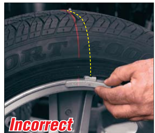
Angle errors from even slight misjudgment of the TDC location lead to an inferior and time-consuming balance with excessive checkspins.
