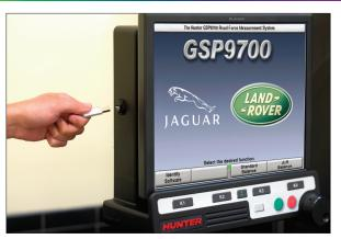
All specifications, TSBs and additional data are stored on an easy-to-use flash thumb drive that plugs directly into a USB port mounted near the LCD screen. Periodic updates are available online through a secure website. To update information, simply download the files onto the thumb drive from any shop computer and plug it into the balancer.
