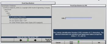
Gaining access to vehicle- and wheel-specific data is as easy as searching for the make and model or entering the VIN on the recall specifications screens...
