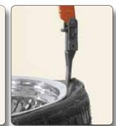
Patented tool head inserts itself into tire, pulls bead over and demounts in one fluid down/ up motion.
