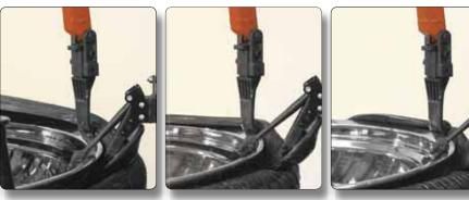
Thin, broad head alleviates stress on the bead, while remaining strong enough to withstand the huge forces created by the most difficult tires.
