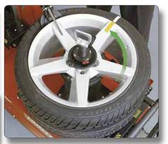
Match-mounting the stiffest point on a tire to the low spot on a rim makes the assembly roll as round as possible.
