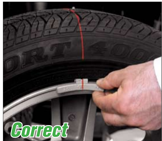
Precision wheel weight placement is fast and easy using the TDC laser as a guide.
