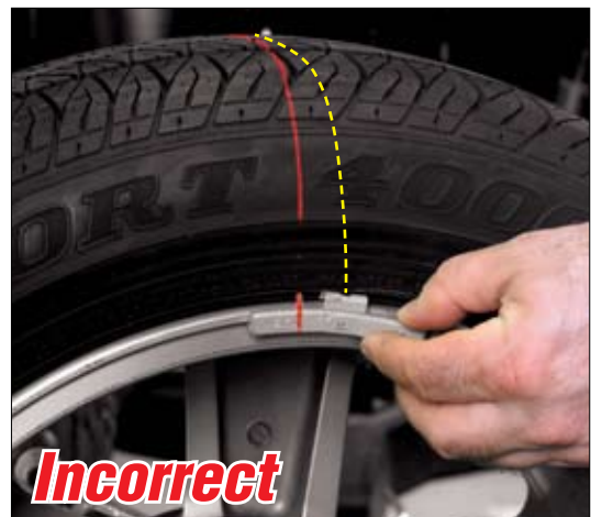
HammerHead TDC Laser reduces weight placement errors by eliminating misjudgment of the TDC position, which often occurs using other methods. Such visual errors lead to an inferior and time-consuming balance with numerous checkspins.
