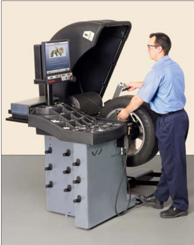
VAS6230A shown with optional printer and printer support kit (VAS6230A/1) and factory installed wheel lift option (VAS6230A/2).
