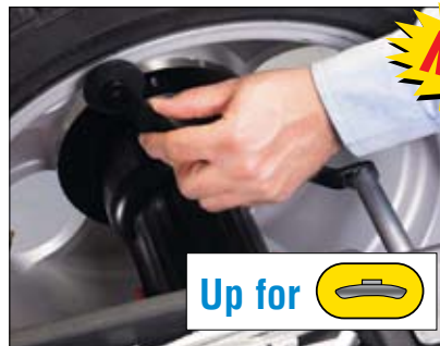
When the technician places the Inner Dataset® arm up on the wheel rim, the balancer automatically selects the "Clip Weight Mode."
