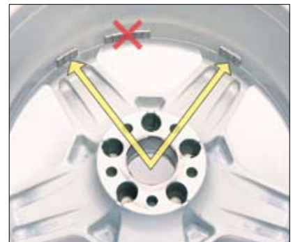
When the technician places the Inner Dataset® arm down inside the wheel, the balancer automatically selects the "Tape Weight Mode."
