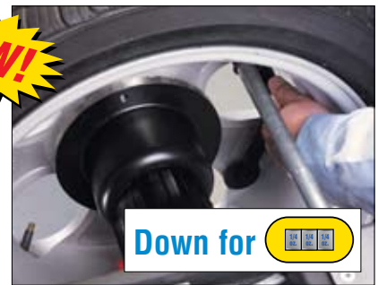
When the technician places the Inner Dataset® arm down inside the wheel, the balancer automatically selects the "Tape Weight Mode."
