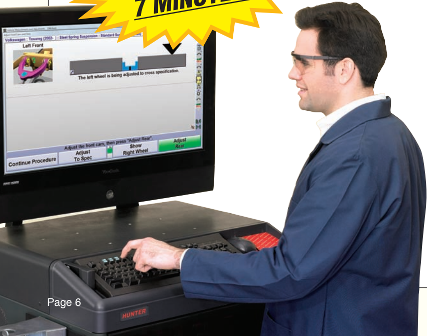
Display for adjusting front slot on left side to match right side cross specification.
